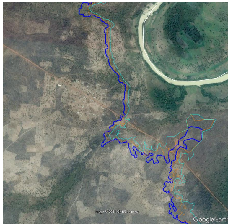
Figure 6-20 : Flooding of the road alongside Sariba (Q1 in light blue, Q10 in orange and Q100 in dark bkue)
