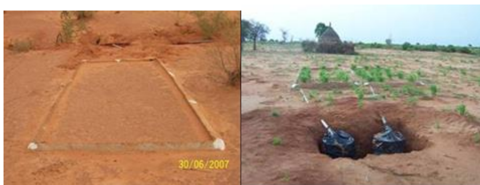
Figure 8-2 : Example of single tank erosion monitoring plots
